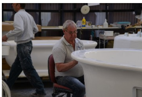
Venus Pool being built by hand at our factory
